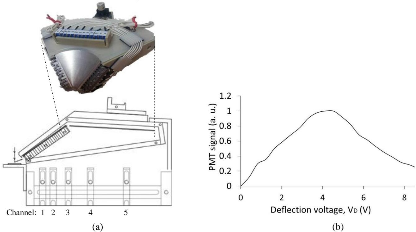
**Figure 6.** PRMA prototype designed for the SEM and a schematic of its detection system. (a) Photograph of the PRMA prototype with energy channel 1 to 5; (b) Experimental analyzer signals obtained in a SEM.
