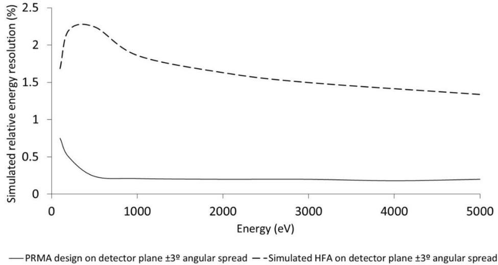
**Figure 3.** Simulated relative energy resolution for the PRMA design as a function of energy in comparison with the HFA for a polar angular spread of  $\pm 3^\circ$ .
