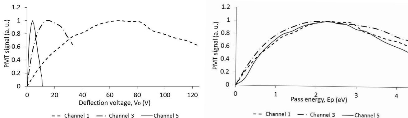
**Figure 7.** Preliminary experimental results from 3 different representative channels along the dispersion plane. Left: PMT signal as a function of deflection voltage,  $V_D$  (V); right: PMT signal as a function of pass energy,  $E_p$  (eV).
