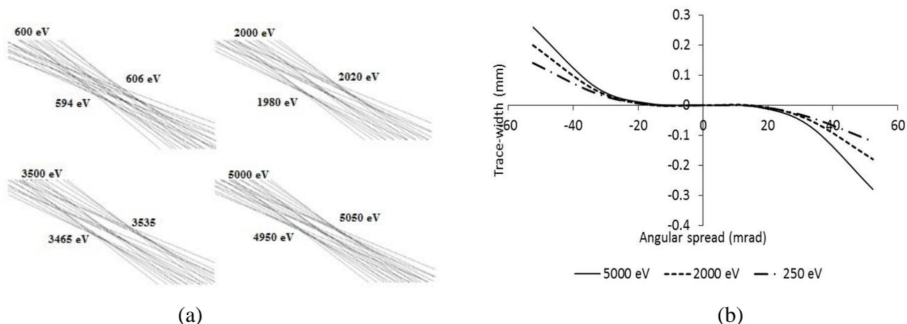
**Figure 2.** Simulated characteristics on the focal plane at selected energies of the PRMA design, for an angular spread of  $\pm 3^\circ$  in uniform steps of  $1^\circ$ : (a) Trajectory paths with energies at  $\pm 1\%$  below and above the central energies of 600, 2000, 3500 and 5000 eV; (b) Trace-width as a function of polar angular spread on the Gaussian focal plane at selected energies. The polar angular spread ranges from  $-3^\circ$  to  $+3^\circ$ .
