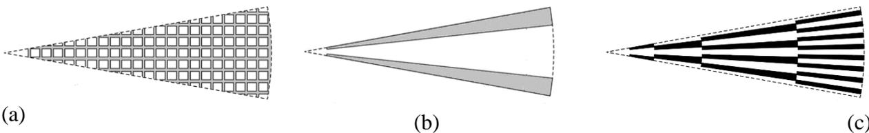
**Figure 4.** Schematic diagram of 3 possible exit grids design (not drawn to scale): (a) Square grid design; (b) Radial slot design; (c) Layered radial slot design.
