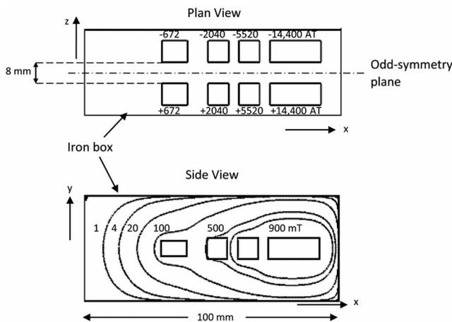
FIG. 2. Simulated field distribution simulation of the Gaussian field analyzer box. Dotted lines indicate contours of equal magnetic field strength along the central odd-symmetry plane.
