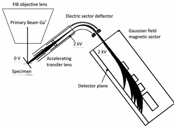
FIG. 5. FIB-SIMS mass analyzer attachment layout.
