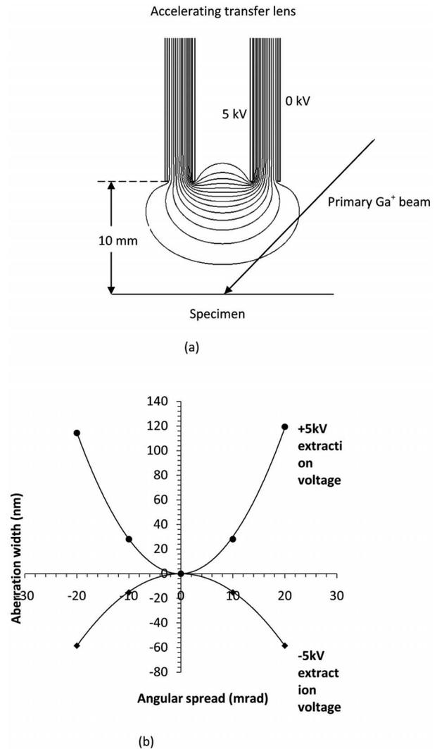
FIG. 9. Simulation of the fringe field effect created by a  $\pm 5$  kV extraction voltage on a 20 keV gallium ion primary beam: (a) simulated equipotential lines of the fringe field in uniform steps and (b) simulated trace-width at the specimen as a function of angular spread in the primary beam.
