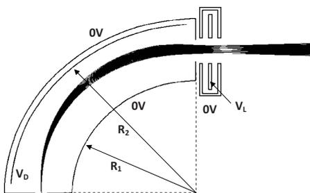
FIG. 6. Simulated ion trajectories through the electric sector designed to compensate for energy dispersion. Nine trajectories are plotted in uniform steps in the angular spread range of  $-25$  to  $25$  mrad, at the energies of 1940, 2000, and 2060 eV ( $\pm 3\%$  spread around the pass energy).
