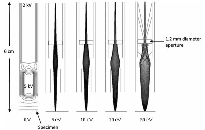
FIG. 7. Simulation of the accelerating transfer lens with a 1.2 mm diameter aperture.
