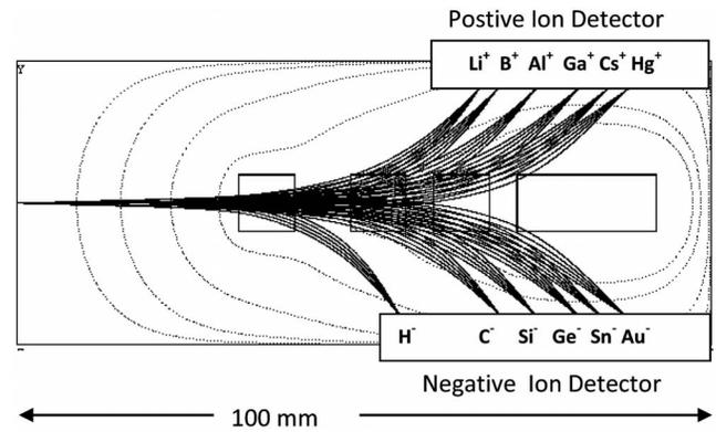
FIG. 3. Simulated 2 keV ion trajectories through the Gaussian field analyzer box design with an input angular spread ranging from  $-25$  to  $25$  mrad.
