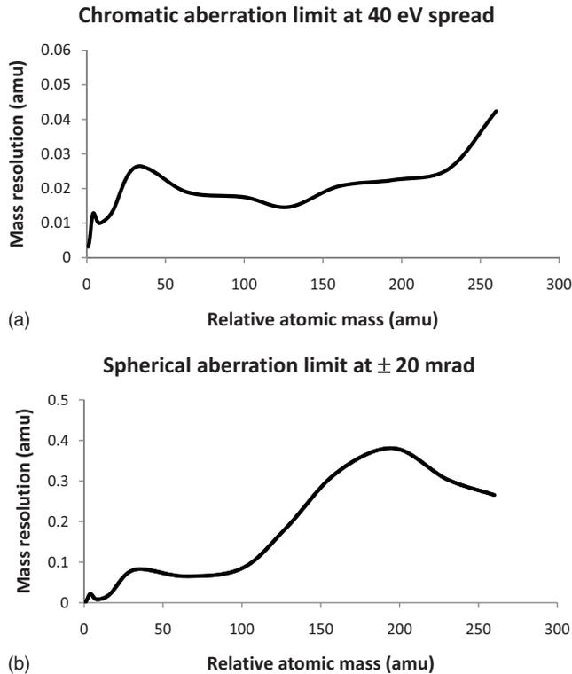
FIG. 8. Simulated mass resolution of the Gaussian field analyzer box design: (a) chromatic aberration limit at 40 eV energy spread and (b) spherical aberration limit for an angular spread of  $\pm 20$  mrad.
