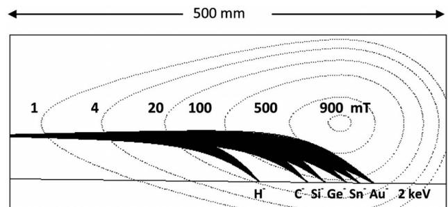
FIG. 1. Simulated ion trajectories through an analytical asymmetric Gaussian magnetic field distribution. The source is located 5 cm from the left hand edge of the diagram; ions have an energy of 2 keV and an angular spread of  $\pm 25$  mrad. The dotted lines indicate contours of equal magnetic field strength (pointing normal to the page).
